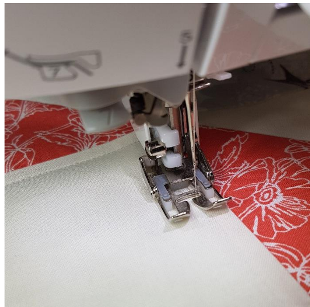
Figure 4 Quilting 1/4 inch away from the seam with a walking foot.
